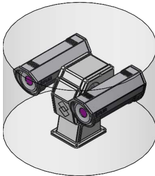
Figure 9.2 FLIR G300 pt series camera exclusion zone. Height 480 mm (18.9"), diameter 740 mm (29.1").
