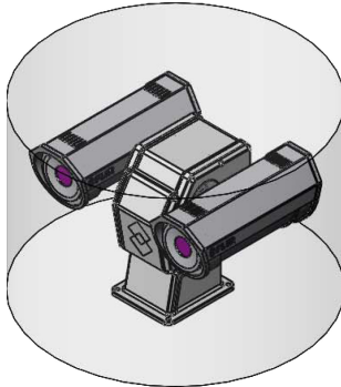
Figure 8.2 FLIR A3xx pt series camera exclusion zone. Height 480 mm (18.9"), diameter 740 mm (29.1").
