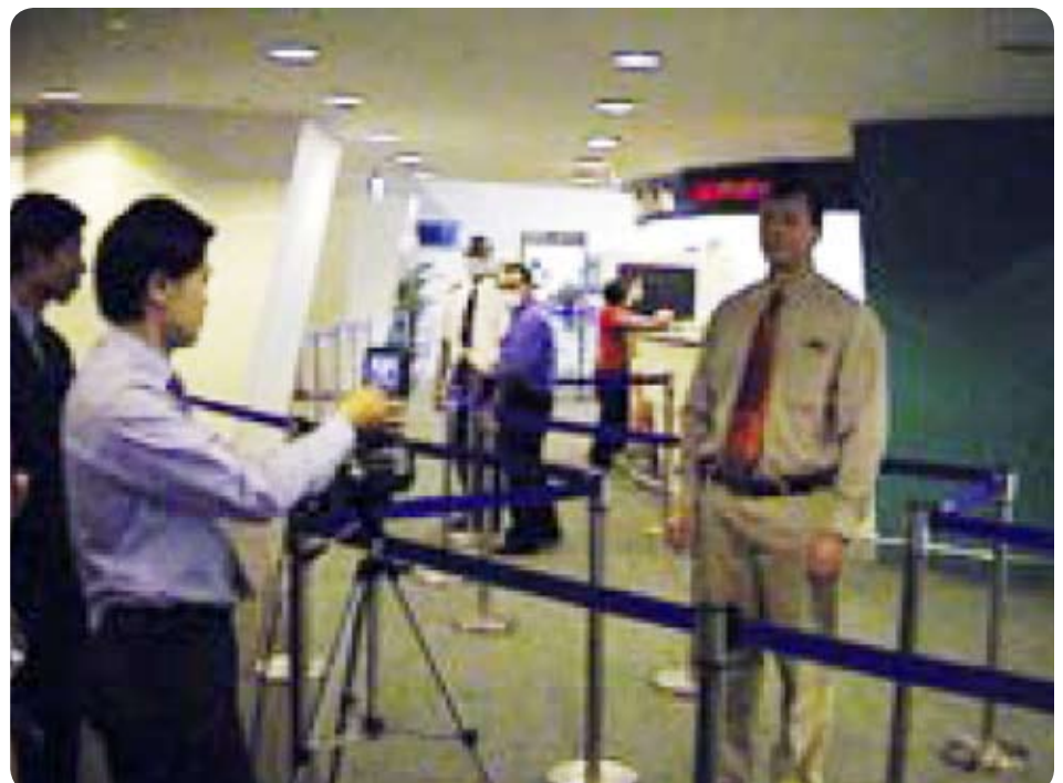
Setting up a ThermoCAM with Automatic Temperature Compensator (ATC) for elevated body temperature detection
