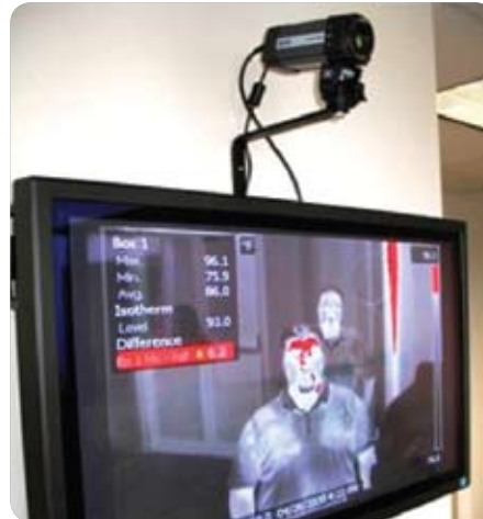
Fixed-mount A320 w/full thermal "color alarming" in progress.
